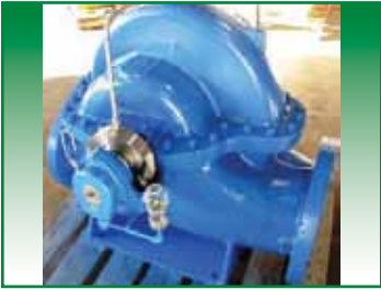
Split Case Repair
